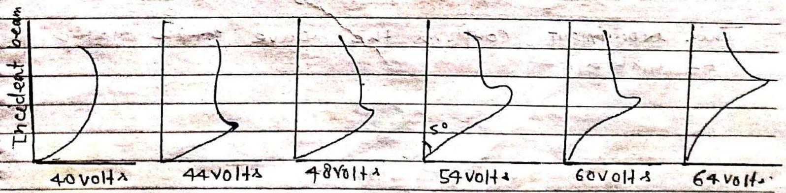
The pronounced current <sup>peak at</sup> ~~peak at~~ 54 volt and at  $50^\circ$  provide ~~and~~ evidence that electron were diffracted by the nickel crystal and verifies the existence of electron wave.
